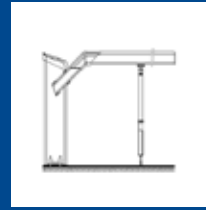
barrier with a hinged catch post
